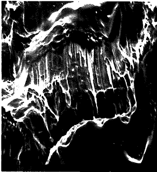
Fig. 8. Creep fracture morphology of Pb–0.09Ca–0.3Sn alloy. Strain softening in creep led to grain fragmentation.
